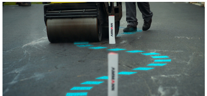
AWR 65-S Walk-Behind Roller with 15° steering angle
